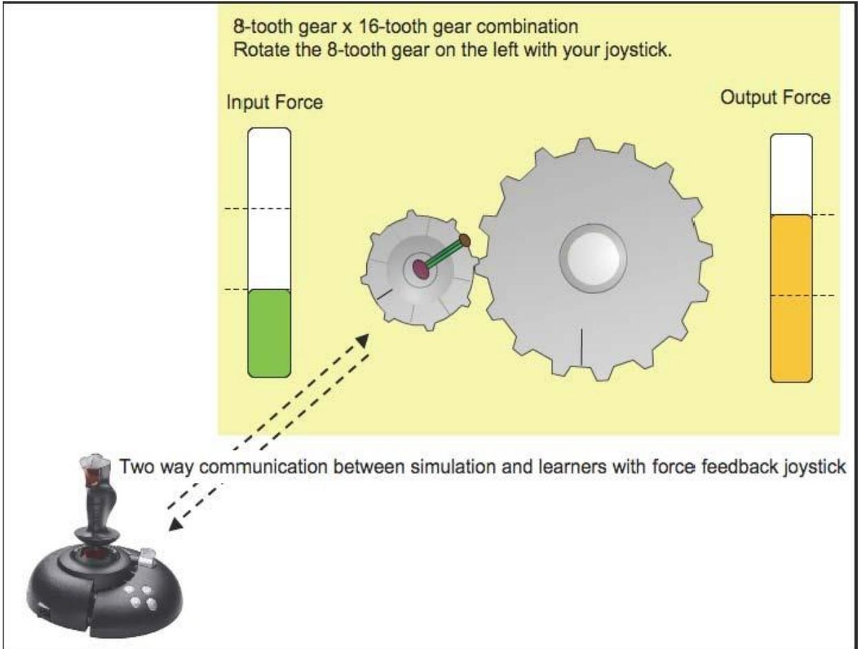
Figure 1 Gear Graphic Simulation with Movement (Joystick and Gears) and Animation with Force Feedback (Joystick)
