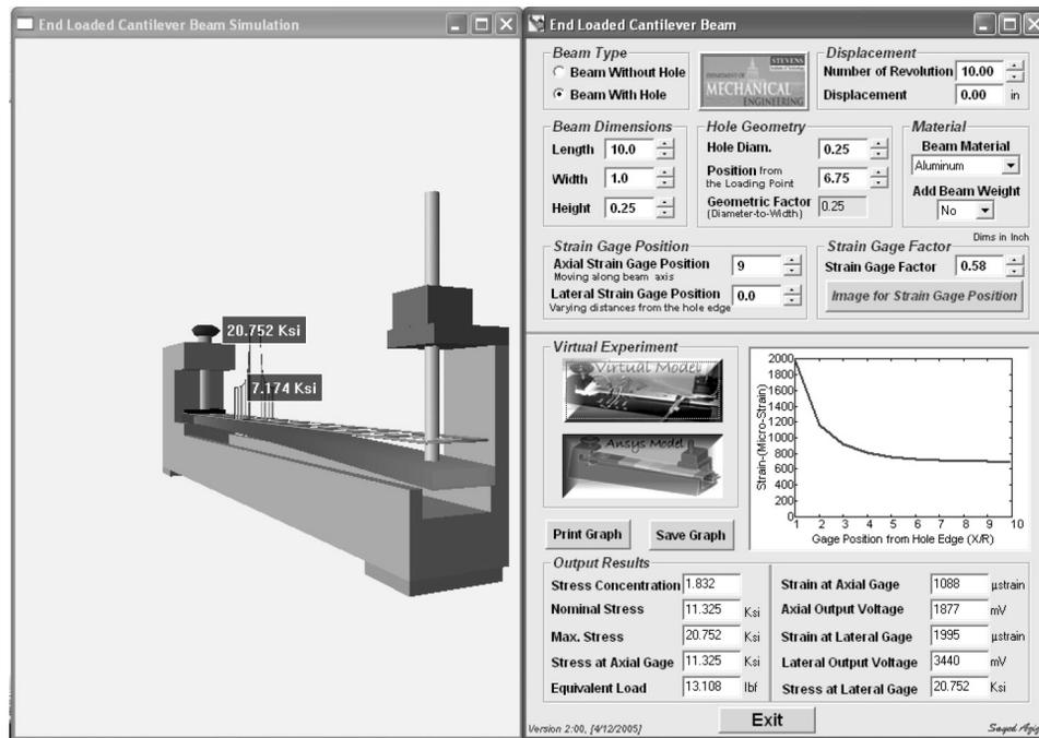
Fig. 4. Stand-alone cantilever beam simulation.
