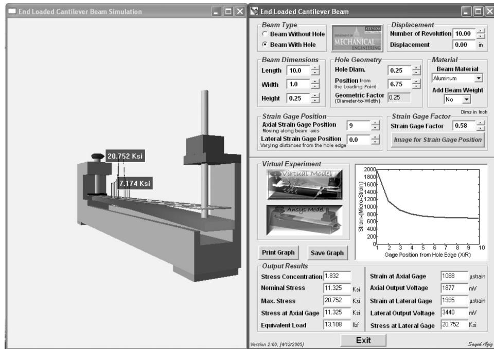
Fig. 4. Stand-alone cantilever beam simulation.
